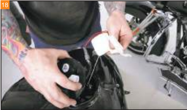
Carefully raise the fuel pump and fuel level sending unit out of the fuel tank spigot.
