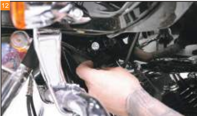
The plastic trim covers on each side of the front tank mounting tabs come off next.
