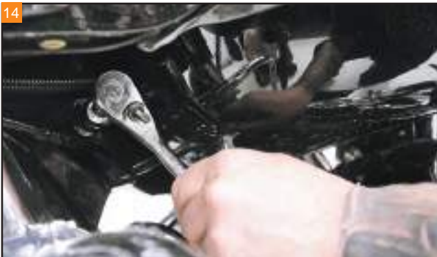
Remove the front mounting bolts with a T40 Torx as well.
