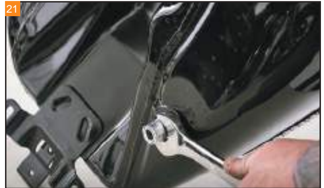
Use a 7/8" wrench to remove the EFI fitting from the bottom left side of the tank.
