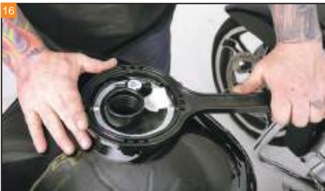
Use the specialty tool to remove the fuel tank lock ring.
