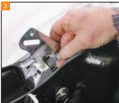
3 The stock grab rail brackets can be removed from the frame. Reinstall the bolt after removing the brackets.
