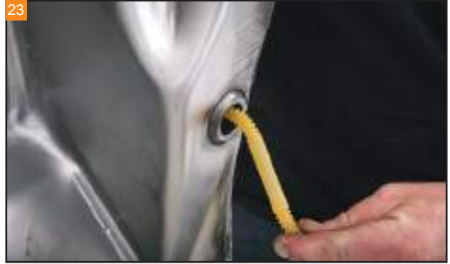
Insert the fuel fitting into the Razorback tank.
