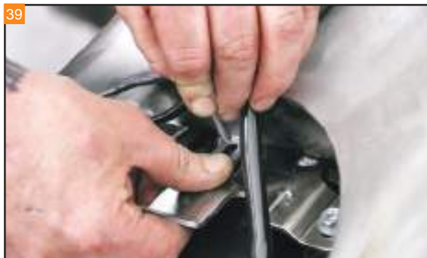
Insert the rear dash-mounting bolt.
