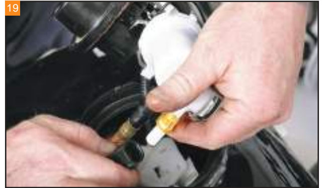
Disconnect the EFI fitting fuel line from the fuel pump.
