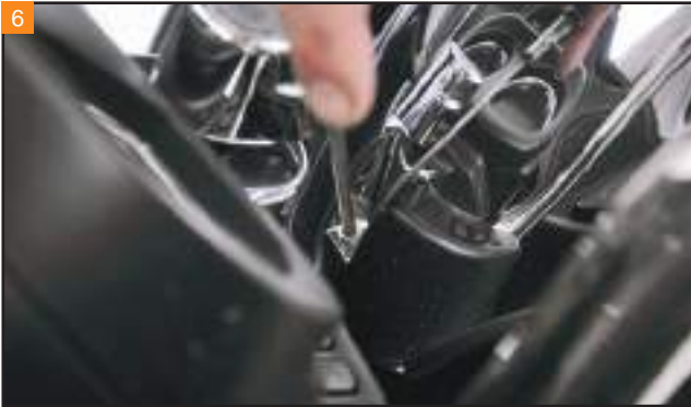
With an Allen wrench, remove the front dash-mounting bolt.
