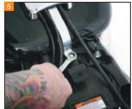
5 Use a 3/8" wrench to remove the lower dash-mounting bolt.
