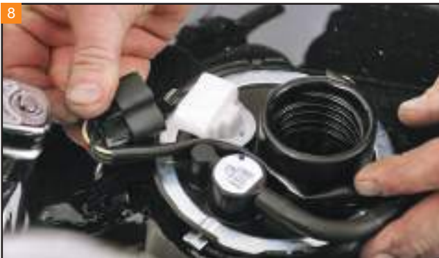
Unplug the wiring for the fuel pump/ fuel level-sending unit.
