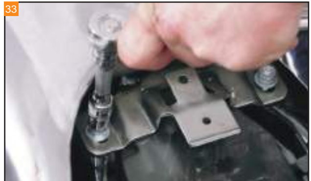
Tighten down all four mounting bolts. Final torque is 15 -20 foot/lbs.
