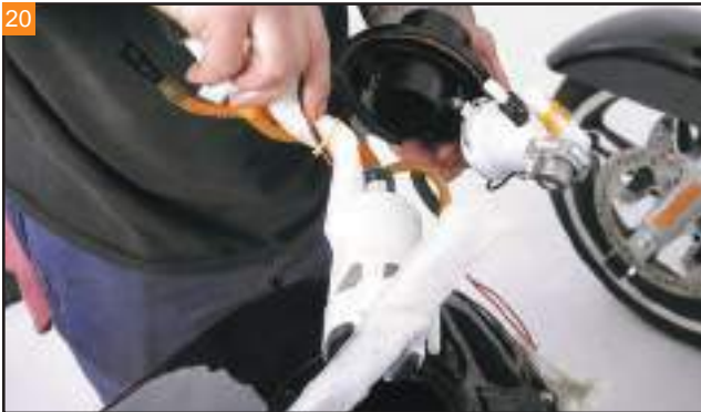
The internals can be removed from the fuel tank.
