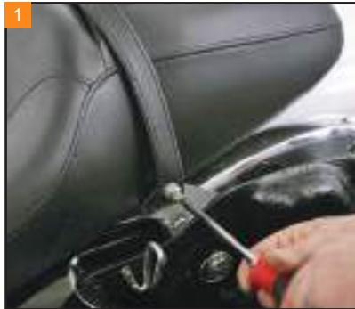
1 With a Phillips screwdriver, remove the seat bolt and bolt for the passenger grab strap.
