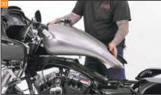
Position the Razorback tank over the back bone.
