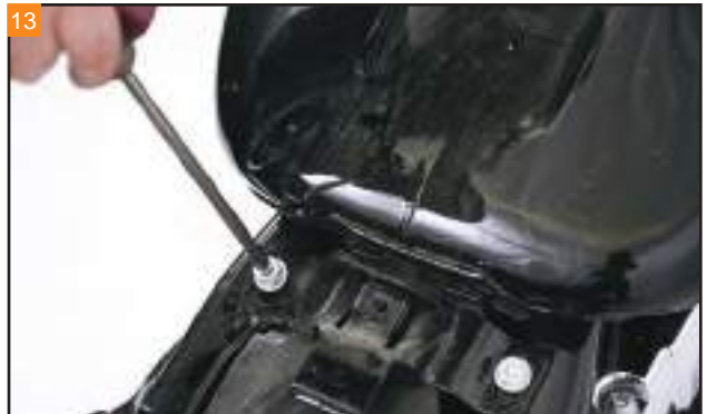
Use a T40 Torx to remove the two rear tank-mounting bolts.
