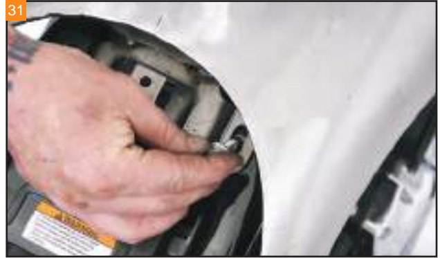
Start the rear tank mounting bolts in the stock location.
