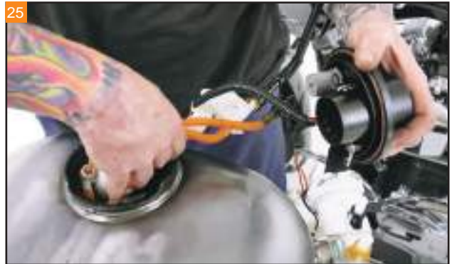
Insert the fuel pump, crossover line, and fuel level-sending unit through the spigot of the Razorback tank.
