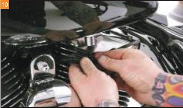
Lift up on the chrome fitting to disconnect the fuel line.
