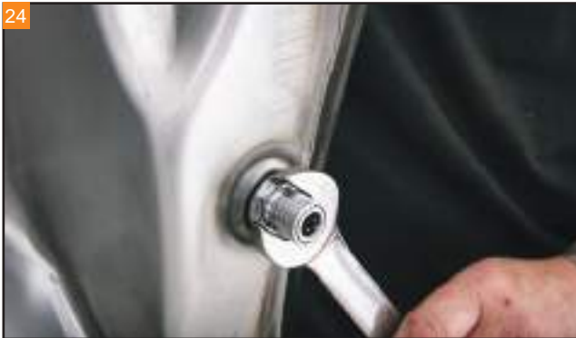
Snug the fitting with a 7/8" wrench.
