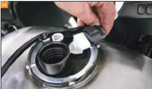
Reconnect the wiring for the fuel pump and level-sending unit.
