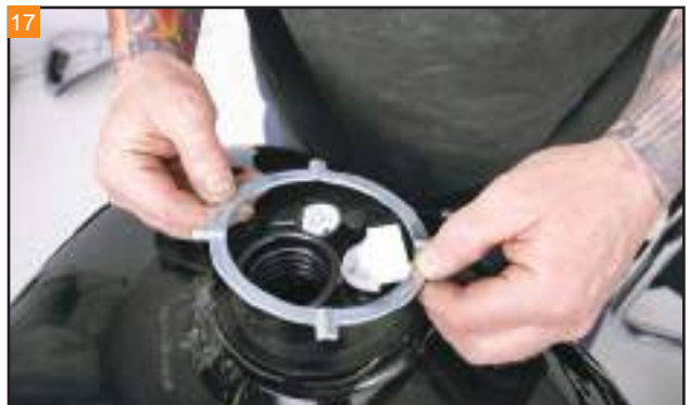
Remove the locking ring from the fuel tank.
