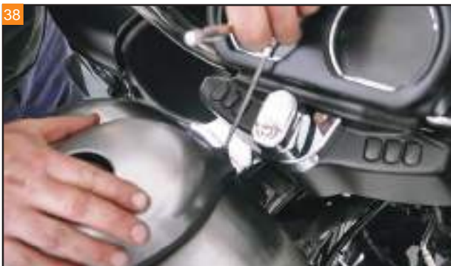
Use an Allen wrench to start the front dash-mounting bolt.
