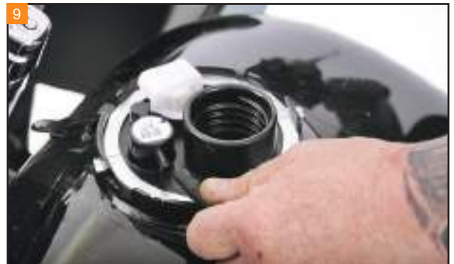
Remove the vent line from the filler neck.
