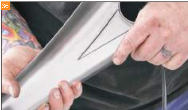
Install the included dash trim onto the new Bagger Nation dash.
