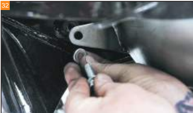
Using the included spacers, start the front mounting bolts.
