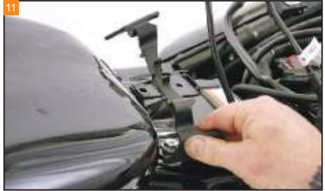
Remove the plastic trim piece from below the tank.
