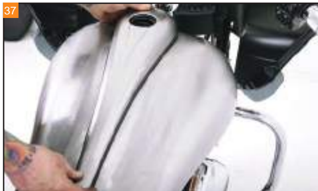
Position the dash over the tank, taking care to ensure the wiring and vent line are both underneath.
