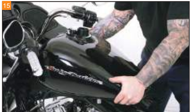
The tank can be lifted up and off the back bone.
