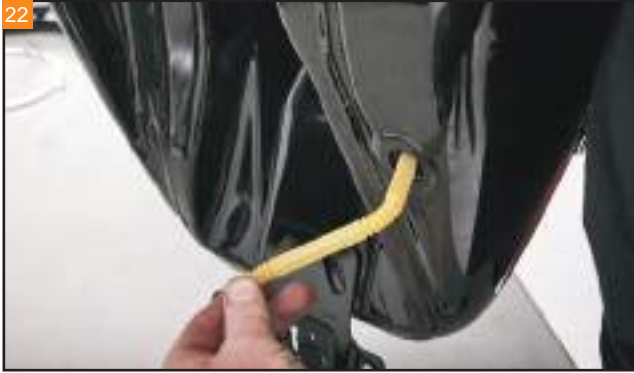
Remove the fuel fitting and line from the threaded hole.
