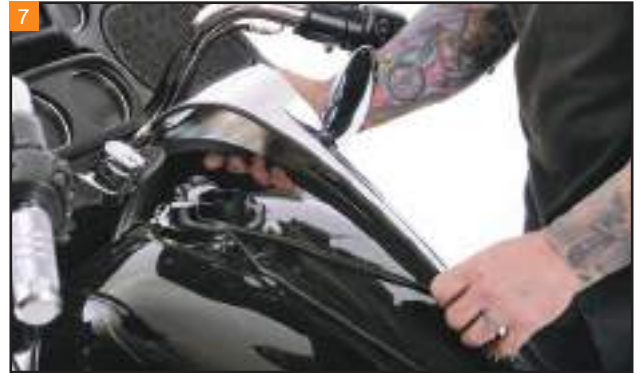
Lift the stock dash up and off the fuel tank. Disconnect the overflow hose from the underside of the dash.
