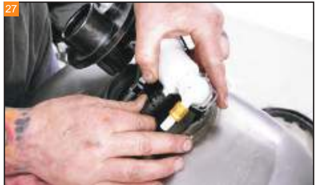
Reconnect the fuel lines to the fuel pump. The two lines are different sizes to prevent error.
