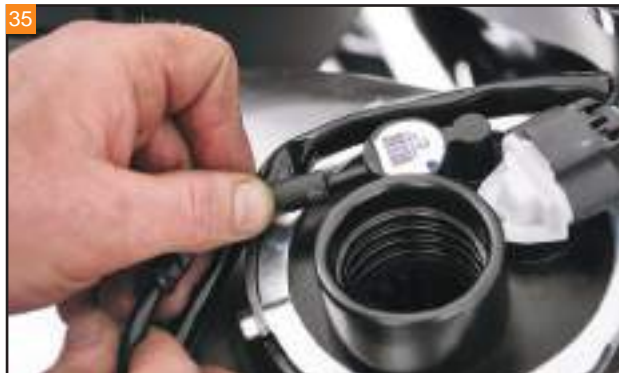
Attach the vent line to the fitting at the fuel filler spout.
