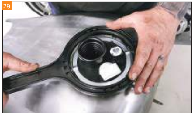
Use the specialty tool to lock the ring into place.
