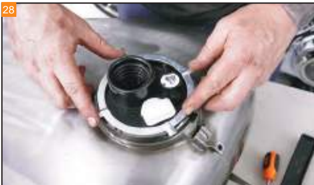
Position the stock lock ring. The ring is marked which side goes up.
