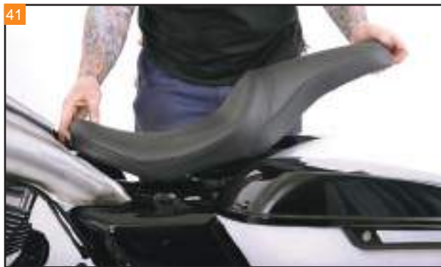
Slide the seat in, catching the mounting tab of the Razorback tank.
