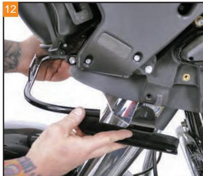
Bring the Bagger Nation Stealth Fairing Support Bar into position at the front of the inner fairing.
