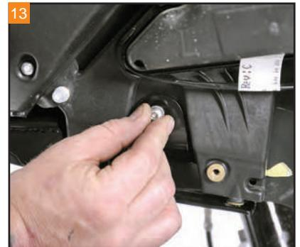
Hold the Stealth Fairing Support Bar in place by loosely installing the stock bolt.
