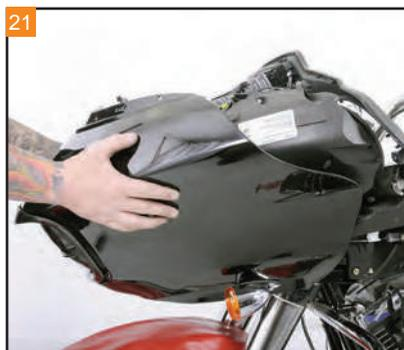
21 Slide the outer fairing back into position.
