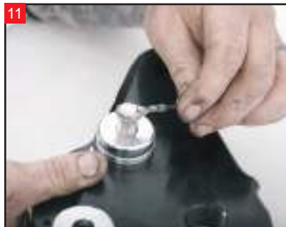
11 Include the stock ground wire on the riser bolt. The other side gets a washer.
