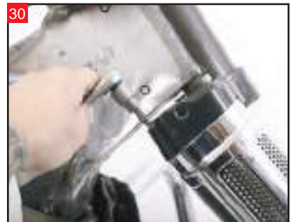
30 Final tighten the bolts in each upper fork slider cover.
