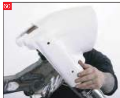
Position the nacelle in place, aligning the pre-drilled holes with the hardware installed on the outside of the triple trees.
