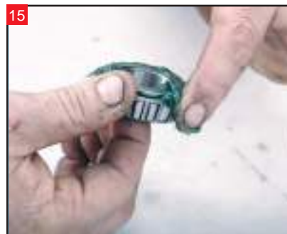
15 Liberally apply bearing grease to the upper and lower neck bearings. A bearing packer is best if available.
