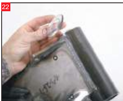
22 The stock upper dust cover will be re-used in this step. Place it over the upper bearing.
