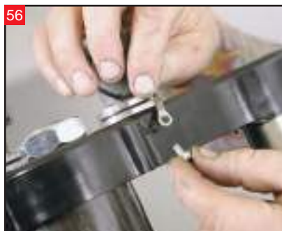
Using thread locker, and then a 5/16" socket, next install the bolt that secures the ground wire for the handlebars.
