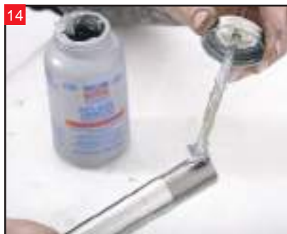
14 Apply a light coat of anti-seize to the neck stem threads.
