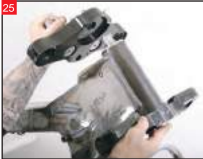
25 Holding the lower tree in place, install the upper triple tree.
