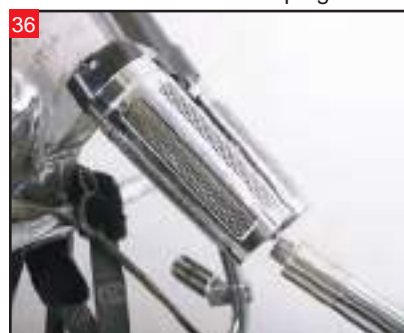
Guide the fork leg into the lower triple tree.
