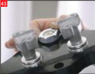
43 Thread the top nut by hand onto the neck stem, where it protrudes from the top tree.
