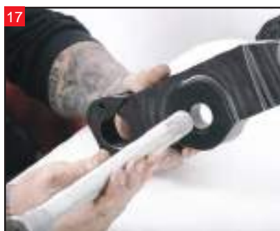
17 From the underside of the bottom triple tree, install the HHI neck stem.
