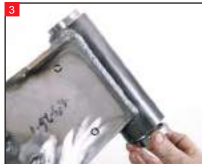
3 Now, insert the lower bearing race, ensuring it is properly oriented.
