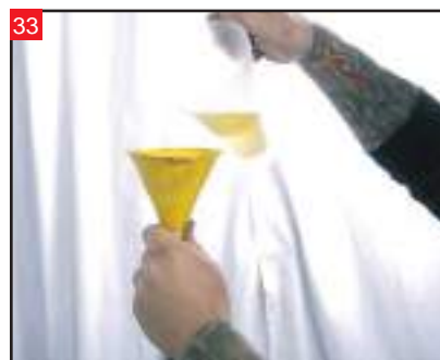
Measure out and add the appropriate grade of fork oil for the application. Then re-install the plug.
