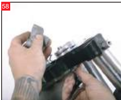
As we are installing a Road King-style raked nacelle, we temporarily remove the risers so the nacelle can slip over the triple trees.
