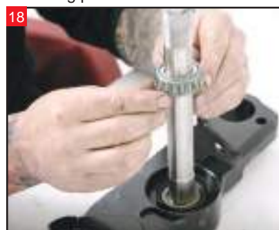
18 First, install the included rubber dust shield, and then the lower Timken bearing on to the neck stem.
