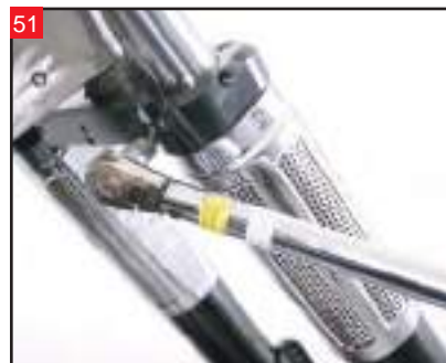
Then final tighten to be 25 ft/lbs of torque. Repeat this process on the other leg.
