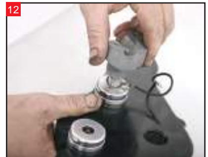
12 Thread the bolt to the stock risers by hand for now.
