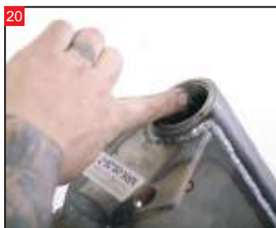
20 Apply a liberal amount of bearing grease to the upper bearing race previously installed.
