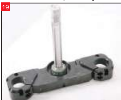
19 The lower neck bearing should bottom out on the lower tree, as seen here.
