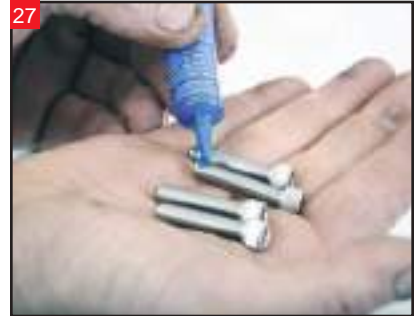
27 Apply a blue thread locker to the included bolts for the upper fork slider covers.
