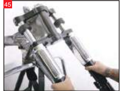
45 Pause and check the range of motion of the front end. You are looking for smooth movement.
