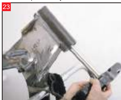
23 Guide the lower tree and neck stem into the motorcycle's neck.
