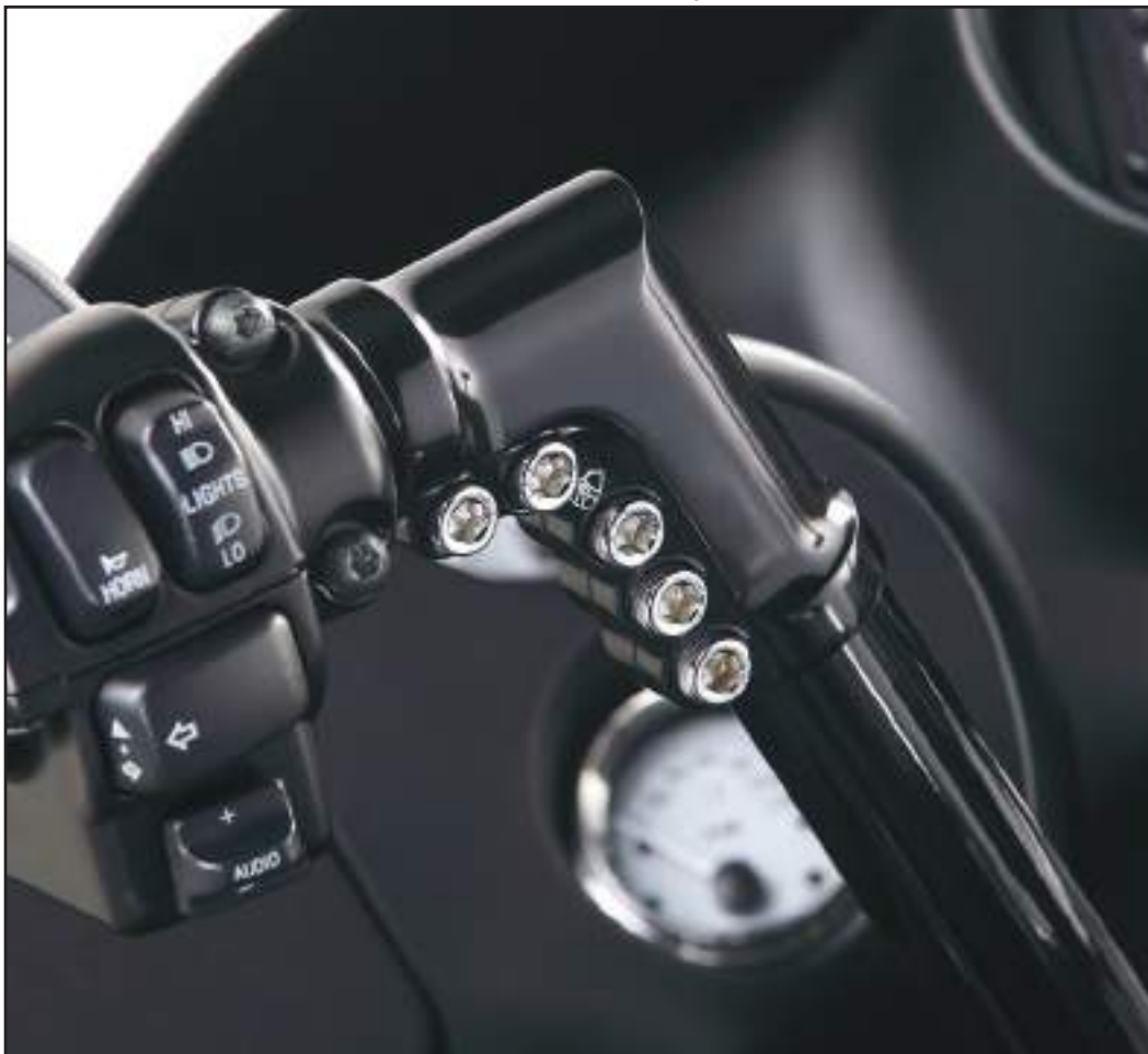
11 Include the stock ground wire on the riser bolt. The other side gets a washer.
