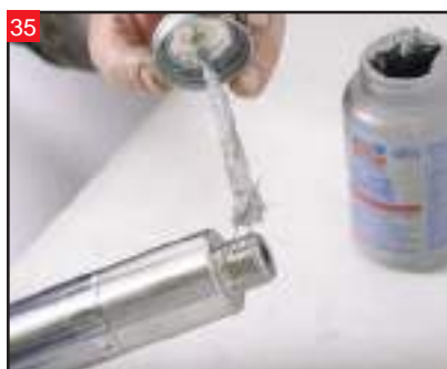
Apply a light coat of anti-seize to the threads of the fork leg extensions.
