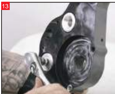
13 Just snug the riser bolts down at this time.
