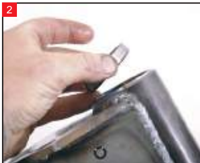
2 Insert the upper bearing race in the new HHI neck. Lightly seat it at this point.
