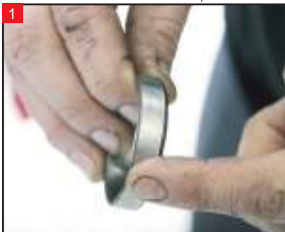
1 We start by applying a very light coat of assembly lubricant to the outer bearing races.
