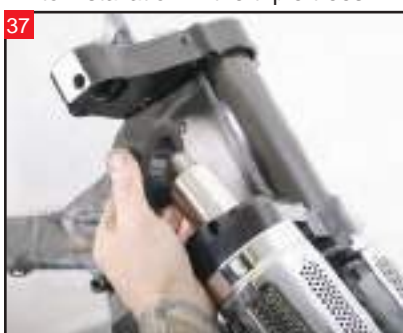
Once through the lower tree, install the rubber ring that serves as the fork stop.
