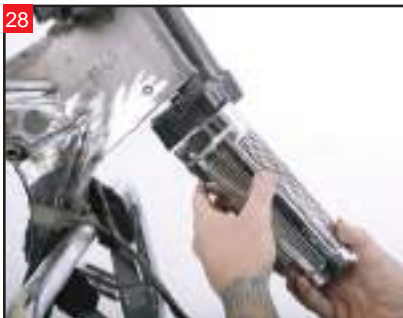
28 Position the upper fork slider in place.
