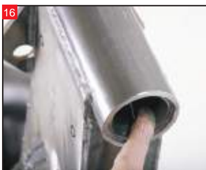
16 Also, apply bearing grease to the lower bearing race you installed in the neck previously.
