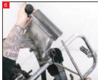
6 Remove the bearing race installer from the neck.
