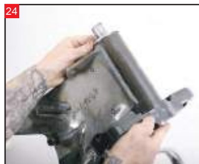
24 Use caution to guide it through the upper bearing and dust cover.
