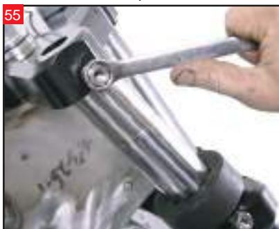
Tighten by hand, and then final torque all four to 15 ft/lbs.
