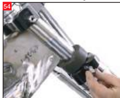
Install the shorter ones in each side of the lower triple tree.
