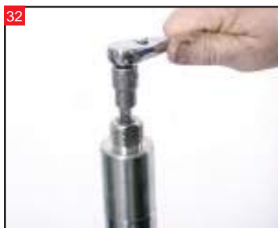
Remove the top plug to gain access to add fork oil.
