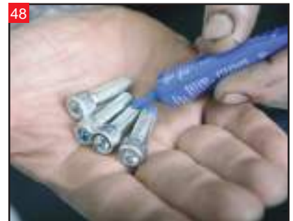
48 Apply thread locker to the four bolts that serve as fork clamping hardware.
