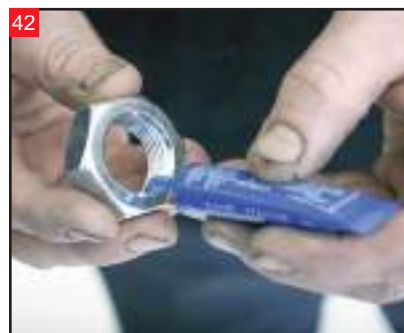
Apply blue thread locker to the top nut.
