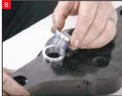
8 Now, install the collar and upper riser bushing in the top triple tree.
