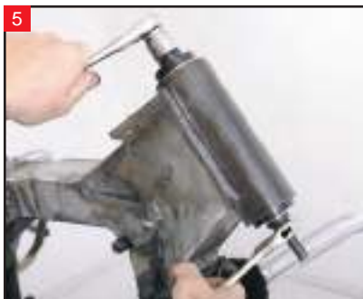
5 Using the rest of the JIMS necking bearing race installer, drive the races in, until they bottom out.
