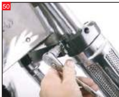
Alternately, tighten the two bolts per side by hand.
