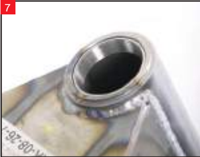
7 The bearing races should be fully seated until they bottom out, as in this picture.
