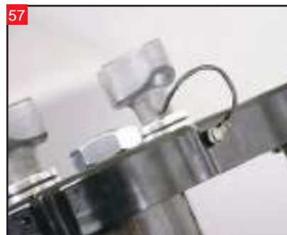
It should be routed with no strain on the wire or terminals.
