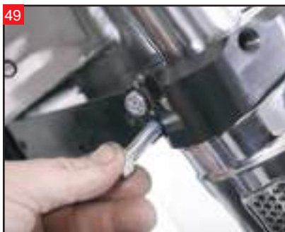
Insert two bolts per side of the lower triple tree.
