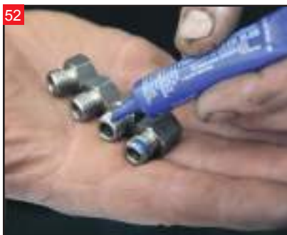
Apply thread locker to the included specialty hardware each side of the triple trees.
