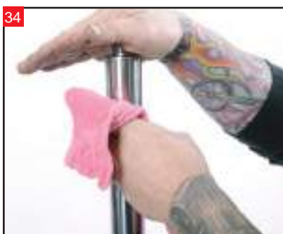
Using glass cleaner, wipe any contaminants from the fork legs prior to installation in the triple trees.
