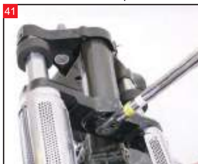
With the legs threaded in place, torque the neck stem to 30 ft/lbs of torque.
