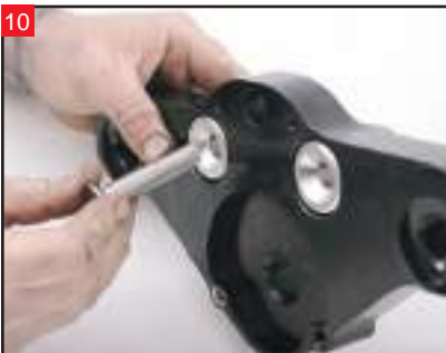
10 Install the included bolts from the bottom of the top triple tree.
