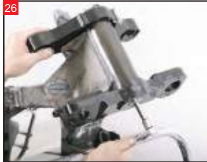
26 Gently thread the neck stem into the upper tree. Tighten the neck stem using a 3/8" ratchet.
