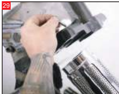
29 Start the bolts in each one by hand.
