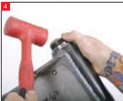
4 Place the JIMS bearing race driver in place, and use a rubber mallet to gently seat the bearings.
