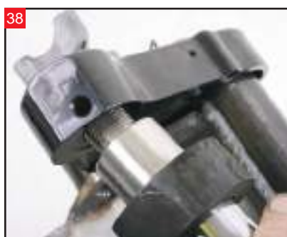
Thread the leg extension into the top triple tree. Go until it bottoms out and stops.
