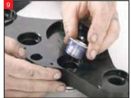
9 Flip the upper tree over, and install the lower riser bushing.
