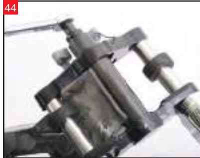
44 Using a 1 1/2" socket, torque the top nut to 80 ft/lbs.
