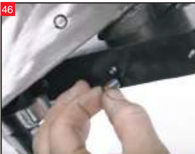
46 Install the set screw in the back side of the lower triple tree. Don't forget to use thread locker on it.
