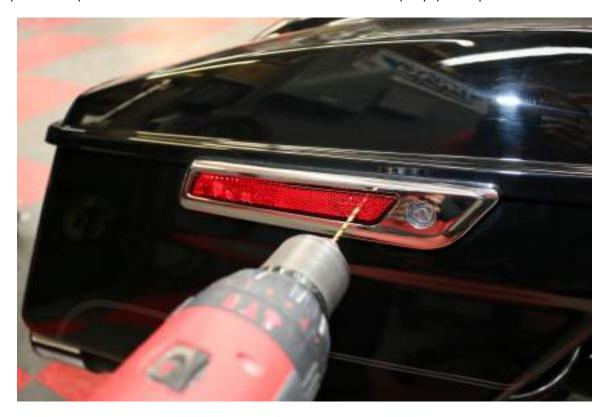
See image below for hole locations. You only need to break through the plastic. Do not drill the hinge cover.
