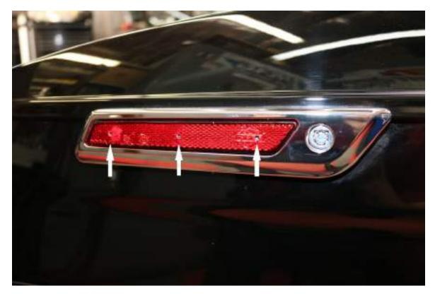
Step 3: Use the provided screws to thread through the reflector.
