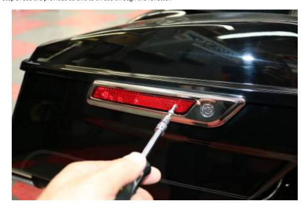
Thread the three screws through evenly,  $\frac{1}{2}$  a turn at a time to push the reflector off of the hinge cover.
