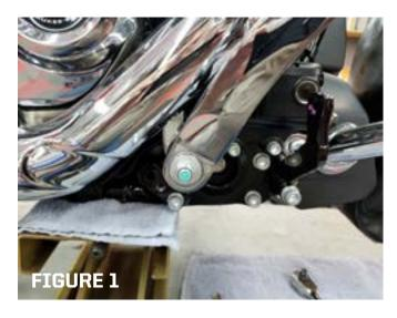
1. Remove right side rider floorboard with rear bracket. (FIGURE 1)
