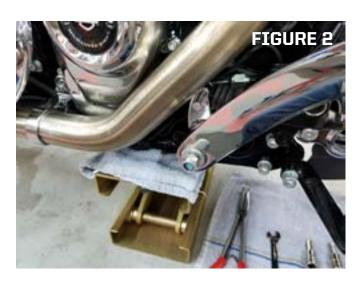
2. Remove front exhaust pipe heat shield & remove cotter pin. (FIGURE 2)
