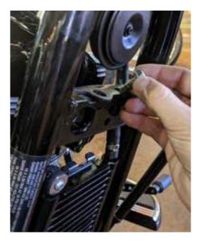
Now you will place the chin scoop mounting plate onto the upper engine mount bracket with the radiused edges facing forward and the threaded inserts facing down.
