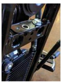
Now you will put the chin scoop in place and install the top two 12-24 fasteners with washers.
