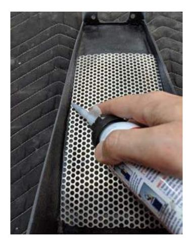
Once the glue is in place, you can secure the grille with a couple pieces of duct tape and an object from around the house to weigh it down while it dries.
