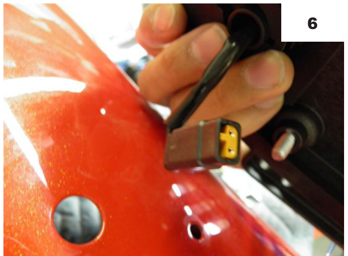
3) Disconnect electrical plug connector and remove stock plate and light assembly from the bike. See Fig #5 /#6
