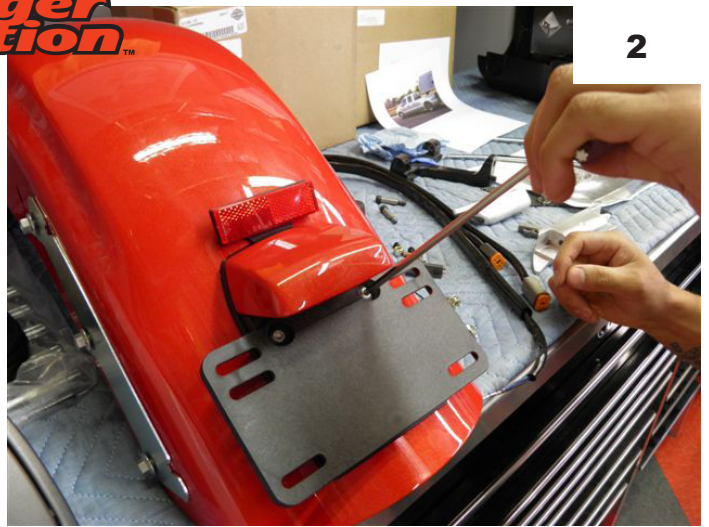
1) The two plate assembly mounting screws are located under your license plate. Remove them. See Fig #1 /#2
