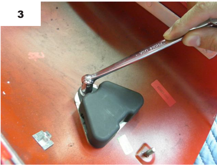
2) On the underside of your fender is a Pyramid shaped plastic box that is retained by one 7/16" nut. Remove this nut and the plastic box. See Fig #3 /#4
