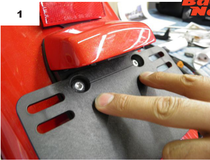
1) The two plate assembly mounting screws are located under your license plate. Remove them. See Fig #1 /#2
