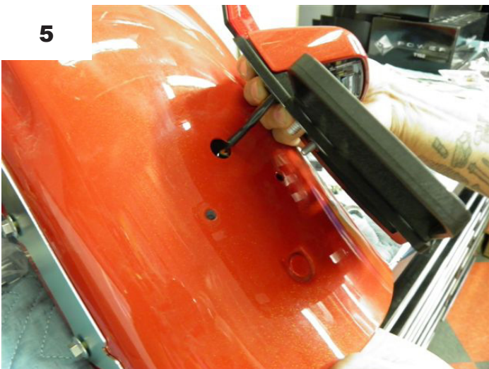
3) Disconnect electrical plug connector and remove stock plate and light assembly from the bike. See Fig #5 /#6
